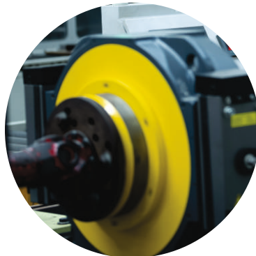
On-load PMSM testing
